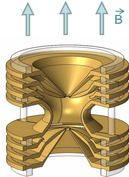
The free cyclotron frequency is inverse proportional to the mass of the ion!
